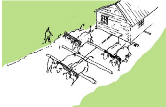
Schematic view: Positioning of Yuntas, and rolling trunks under the house
